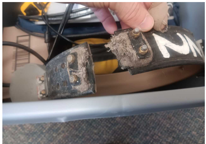
"Caspers" collar showing the cotton layer that rotted off
