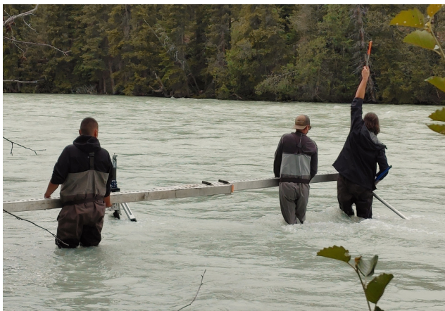
Photos: TNG Fisheries crew installing the SONAR system in the Taseko River to count vulnerable Taseko Ts'eman (sockeye).
