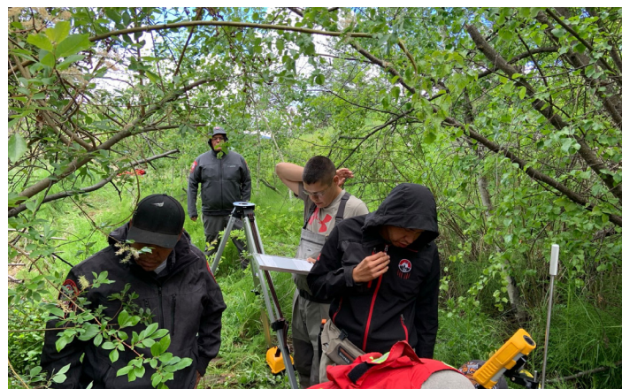
Photo 6: TNG Fisheries Field Coordinator Leonard English and Fisheries Technician Winston Bambrick, TNG Rangers Jimmy Harry and Jason Hance, and hydrologist Derek Brzoza measuring water discharge at Hanceville using an acoustic Doppler velocimeter (ADV) – part of our Water Quality and Quantity Monitoring Program, and to support future hatchery work at Hanceville.
