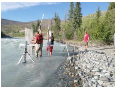
Pics 3, 4 and 5 (above) – Taseko Sonar site – set up of diversion fence and ARIS (sonar) for under water visuals of salmon migrating up the Taseko River to either Elkins Creek or Taseko Lake. Mason Seaward, Jason Hance, Jimmy Harry, Paul Grinder and Wacey Alphonse assisting in set-up of fence. Sonar set up by Leonard English.
